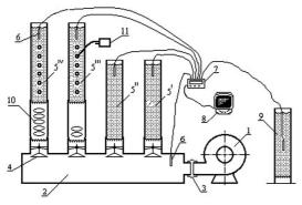
**Figure 1.** Schematic diagram of drying test rig: 1 - air blower;  $2 - chamber with constant static pressure; <math>3 - flexible joint; 4 - restrictor; <math>5^{I}, 5^{II}, 5^{II}, 5^{IV} - ventilated cylinders with grain; 6 - temperature sensors and moisture content; 7 - secondary ALMEMO measurement unit; 8 - computer; 9 - natural ventilation cylinder with grain; 10 - ozonators; 11 - measurement unit of ozone concentration.$
